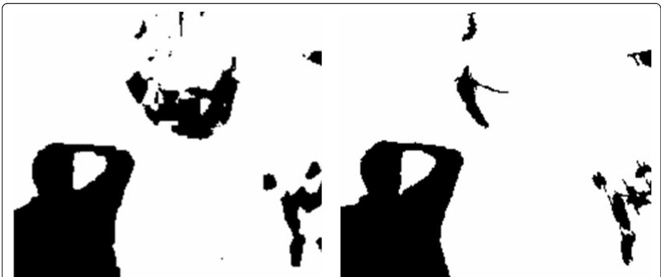
**Figure 4 Comparison of shadow detection results between only using TAM image and after combining intensity image.** Left: Shadow detection result only using TAM image. Right: shadow detection result after combining intensity information.
