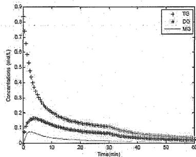
Figure 5. Concentration profiles of TG, DG, MG for two-step reaction
