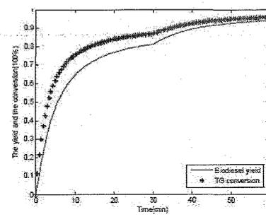
Figure 7. The biodiesel yield and TG conversion profiles for two-step reaction
