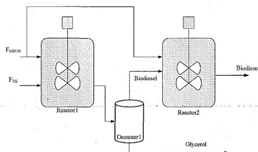
Figure 1. Two-step transesterification reaction system
