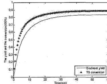
Figure 4. The biodiesel yield and TG conversion profiles for one-step reaction
