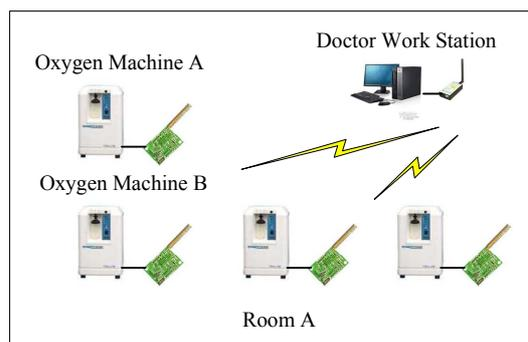
Figure 1. Layout of equipment in a consulting room
