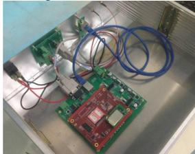
Figure 10. The picture of wireless intelligent gateway
