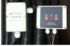
Figure 8. The picture of wireless waterlogging monitoring node
