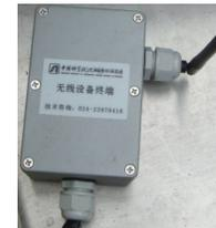
Figure 6. The factual picture of WIA-PA wireless transparent transmission module
