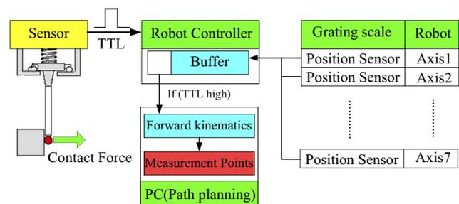
Figure 5 Sketch map of weld joint measurement
