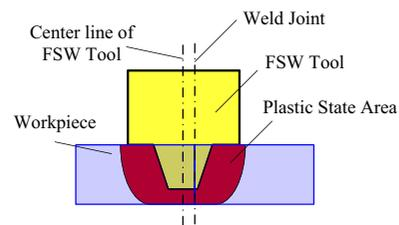
Figure 16 The weld joint measurement process
