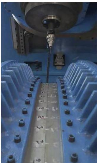
process is controlled manually and animated by the eyes of the controller. When the probe is fixed in the end of the robot contacted with the weld joint, the robot will record the axis positions with the method proposed in Section 3.1.
