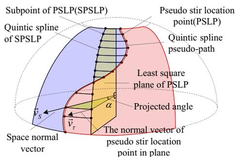
reliable the result is. The parameters  $A, B$  and  $C$  of LSP ( $Ax + By + Cz + I = 0$ ) can be expressed by equation (12) with the coordinate of PSLP  $[Q_1, Q_2, Q_3 [\dots] Q_i (x_i, y_i, z_i) [\dots], Q_n]$ :
