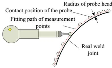
Because the end of the probe is a small ball, the measurement value calculated by forward kinematics is the position above the point on the weld joint with a radius distance in the normal direction of the surface.
