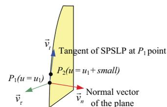
By now, the pseudo FSW tool location points and corresponding normal vectors are calculated. For the pseudo FSW tool location points,  $[Q_1, Q_2, Q_3 \dots] [\dots], Q_n]$  are a radius distance above the real FSW tool location points, it is easy to understand, and the real FSW tool location points  $[P_1, P_2, P_3 \dots] [\dots], P_n]$  can be obtained by equation (16):
