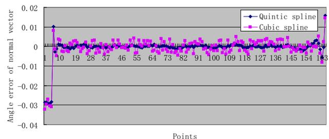
between  $\pm 15 \mu\text{m}$  when the error of the cubic spline is  $\pm 60 \mu\text{m}$ . Most of the angle error of the normal vector direction is controlled at  $\pm 0.003^\circ$ . But, the angle error of cubic spline is larger and is mostly about  $\pm 0.005^\circ$ .
