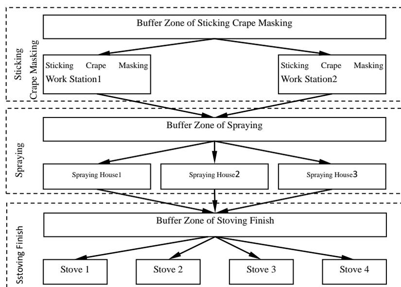
Figure 2 Deployment Diagram of Work Station in Multi-Sticking Crape Masking Procedure
