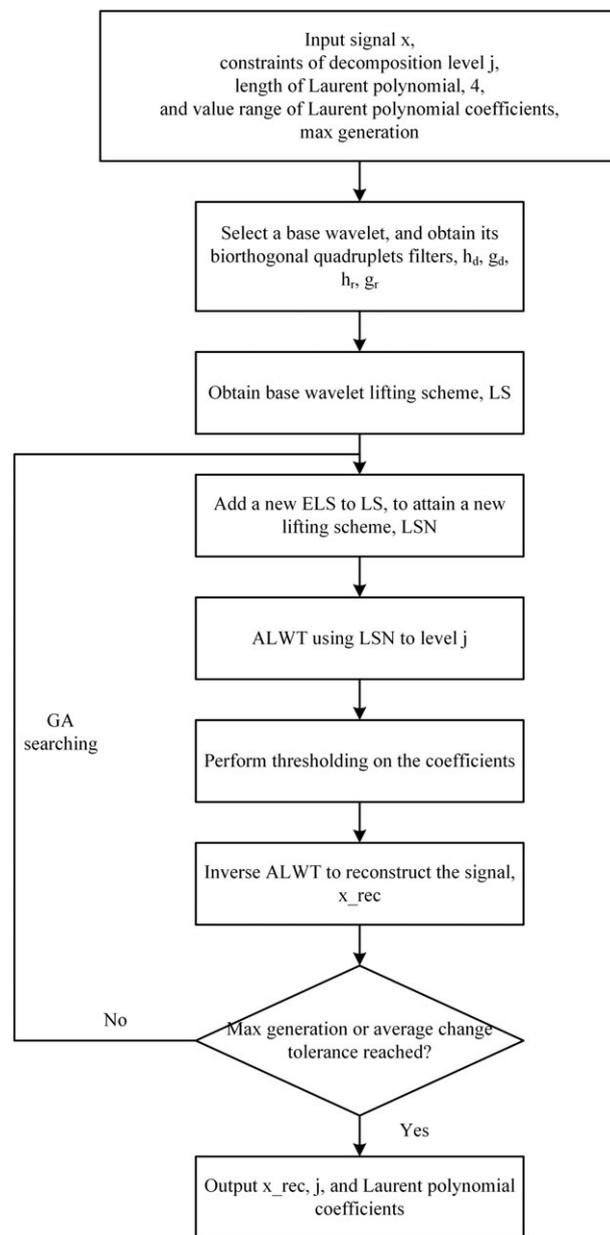
**FIGURE 4** Flowchart of adaptive lifting wavelet transform (ALWT) denoising. GA = genetic algorithm; ELS = elementary lifting step
