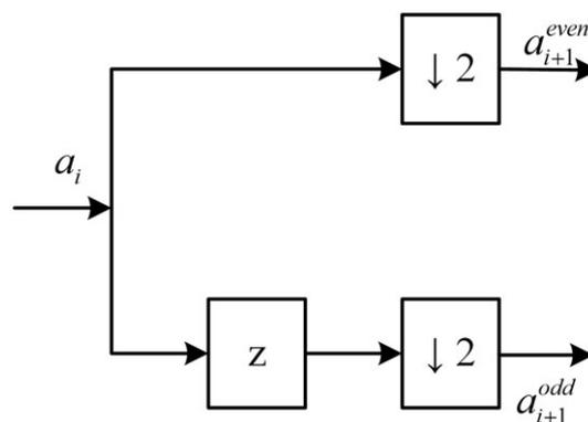
**FIGURE 1** Illustration of lazy wavelet transform (z represents the unit advance operator and  $\downarrow 2$  denotes downsampling by two)
