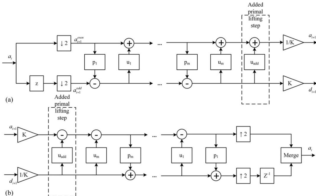
FIGURE 3 Forward and inverse implementations of adaptive lifting wavelet transform (ALWT): (a) forward ALWT; (b) inverse ALWT
