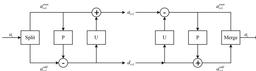
FIGURE 2 A schematic diagram of lifting wavelet transform and inverse lifting wavelet transform
