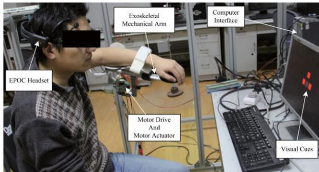
Fig. 3. The setup of the proposed SSVEP-BCI robotic rehabilitation system for upper extremity.
