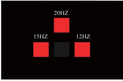
Fig. 2. The design of three visual stimulus. The cues were presented by the square shape, which flashes between red and black at a frequency. The left square flashes by 15 Hz frequency, the top square flashed by 20 Hz frequency and the right square flashes by 12 Hz frequency. The black square in the center represents no flickering frequency.
