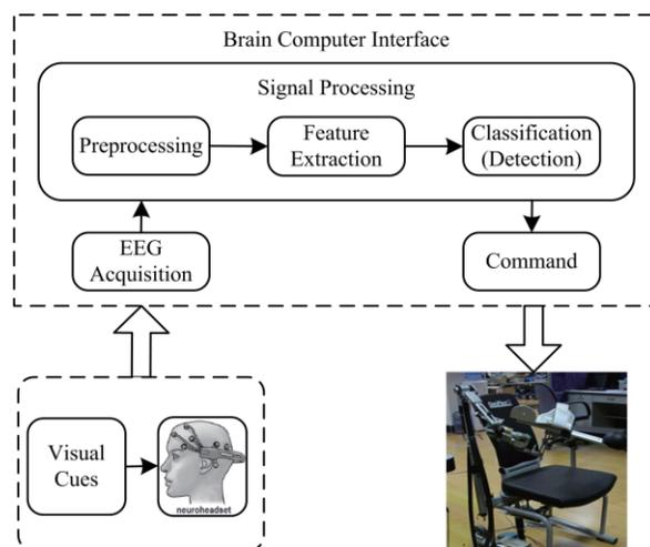
Fig. 1. The framework of the integrated upper extremity robotic rehabilitation system combined with SSVEP-based Brain-Computer Interface (SSVEP-BCI).
