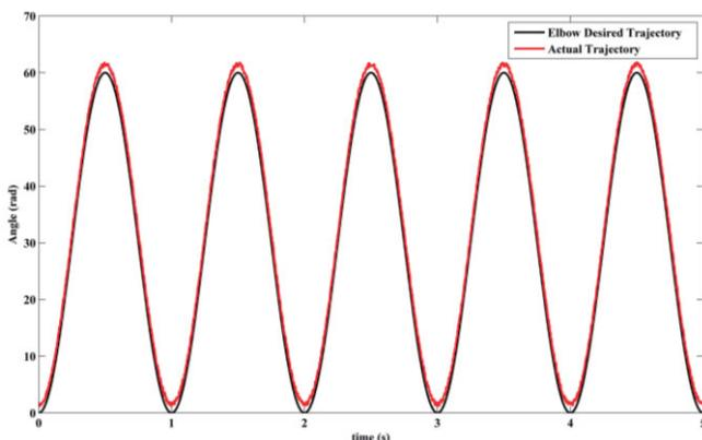
Fig. 5. The trajectory tracking result of medium motor mode (1.0 HZ).
