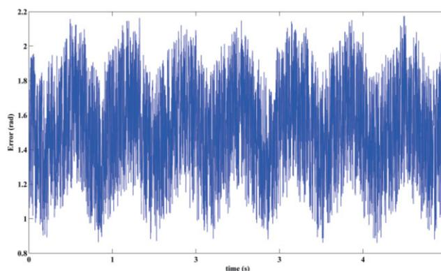
Fig. 9. The tracking error of fast motor mode (1.5 HZ) by the robot.
