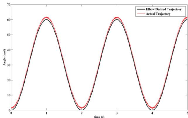
Fig. 4. The trajectory tracking result of slow motor mode (0.5 HZ).
