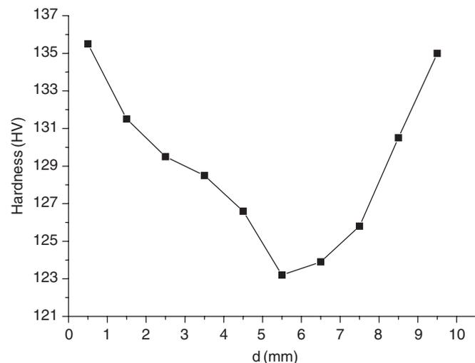
Fig. 13. Hardness distribution in the Z-direction of LMDS-formed thin-wall sample.
