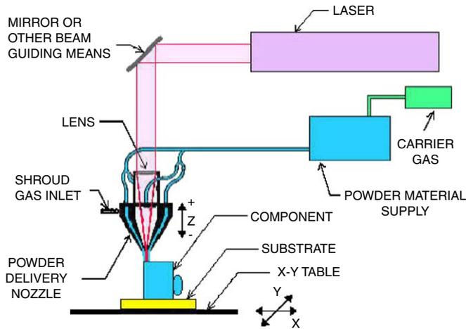
Fig. 1. The diagrammatic sketch of the LMDS system.
