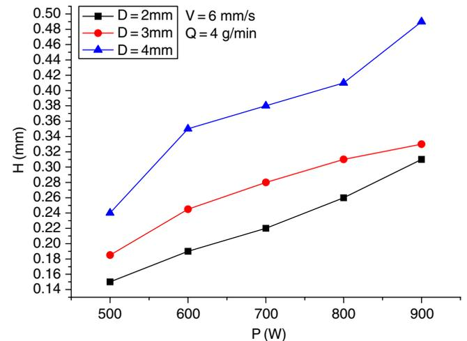
Fig. 4. The influences of laser power and spot diameter on the height of single-cladding layer.
