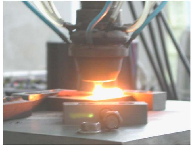
Fig. 2. The working coaxial powder nozzle of the LMDS system.
