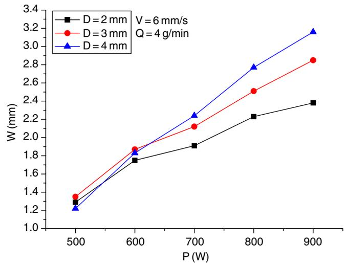
Fig. 6. The influences of laser power and spot diameter on the width of single-cladding pass.
