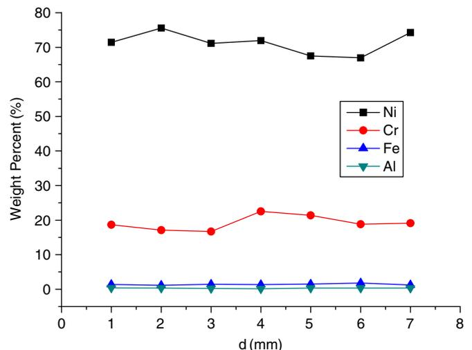
Fig. 14. Composition distribution in the Z-direction of LMDS-formed thin-wall sample.
