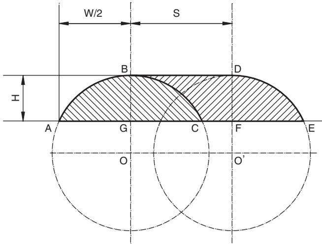
Fig. 7. The schematic diagram of the cross section in the ideal overlapping state.
