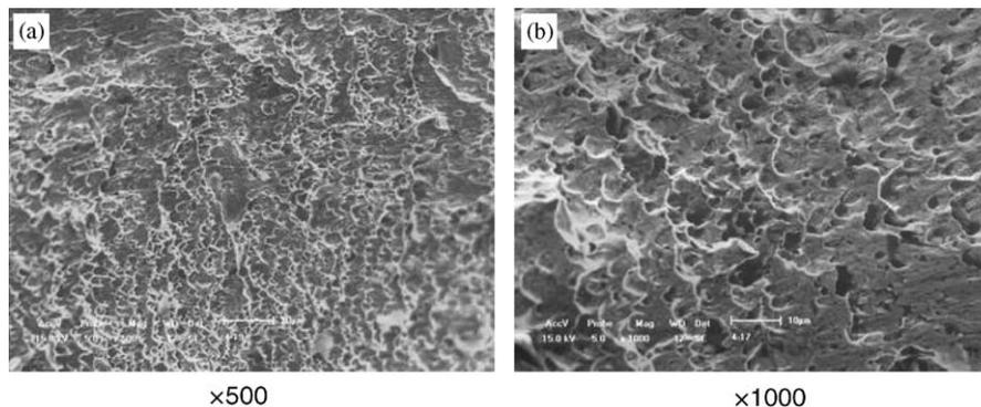
Fig. 12. SEM morphology of tensile fracture surface of LMDS-formed sample.
