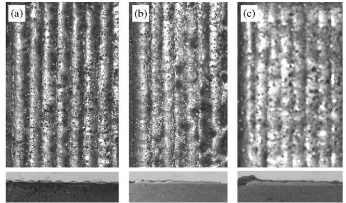
Fig. 8. Appearances of planar scanning experimental specimens. (a) Scanning space 2.1 mm. (b) Scanning space 1.7 mm. (c) Scanning space 1.3 mm.
