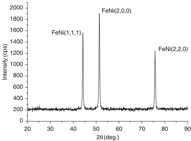
Fig. 11. The X-ray diffraction result of the surface of the nickel-based superalloy cladding layer.
