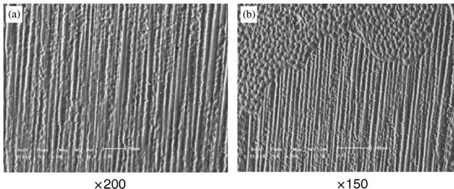
Fig. 10. SEM micrograph of the longitudinal section of LMDS-fabricated sample in the Z-direction. (a) At the middle of cladding layer. (b) At the top of cladding layer.
