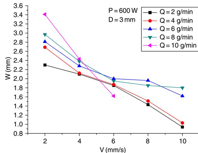
Fig. 5. The influences of powder-feeding rate and scanning velocity on the width of single-cladding pass.
