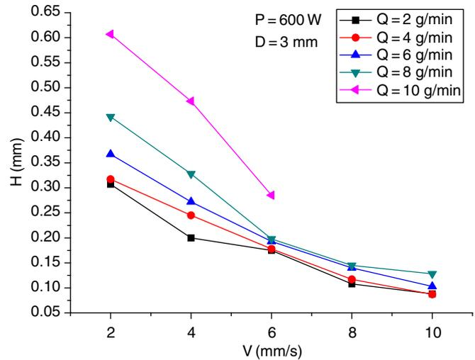
Fig. 3. The influences of powder-feeding rate and scanning velocity on the height of single-cladding layer.
