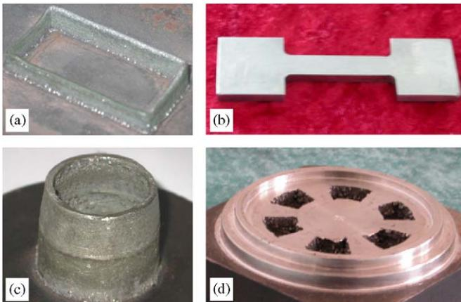
Fig. 9. Nickel-based superalloy components fabricated using LMDS system. (a) Rectangular thin-wall sample. (b) Standard tensile sample. (c) Conical tube sample. (d) Rotary table sample.
