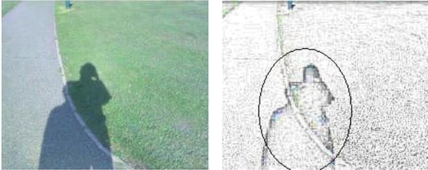
**Fig. 1.** The left image is the original image; the right the enhanced image by Kimmel Retinex Algorithm, inside the ellipse regions of which is strongly illuminated at the center though not brightened correctly at the boundaries
